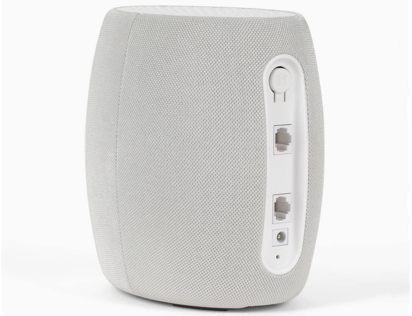
Image: Rear view of a Motorola Q14 router unit, clearly showing the 2.5 Gbps Ethernet port, which enables true multi-gigabit speed.
