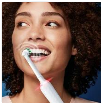
Image 5.2: The 360° visual pressure sensor indicating excessive brushing force.
