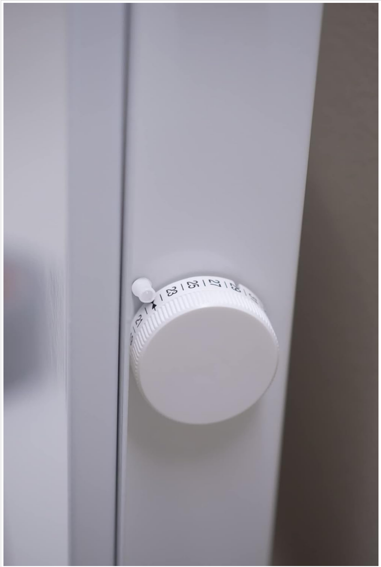
Image 3: Close-up of the rotary thermostat knob on the side of the Adax VP12 H heater. The knob has temperature markings for precise adjustment.
