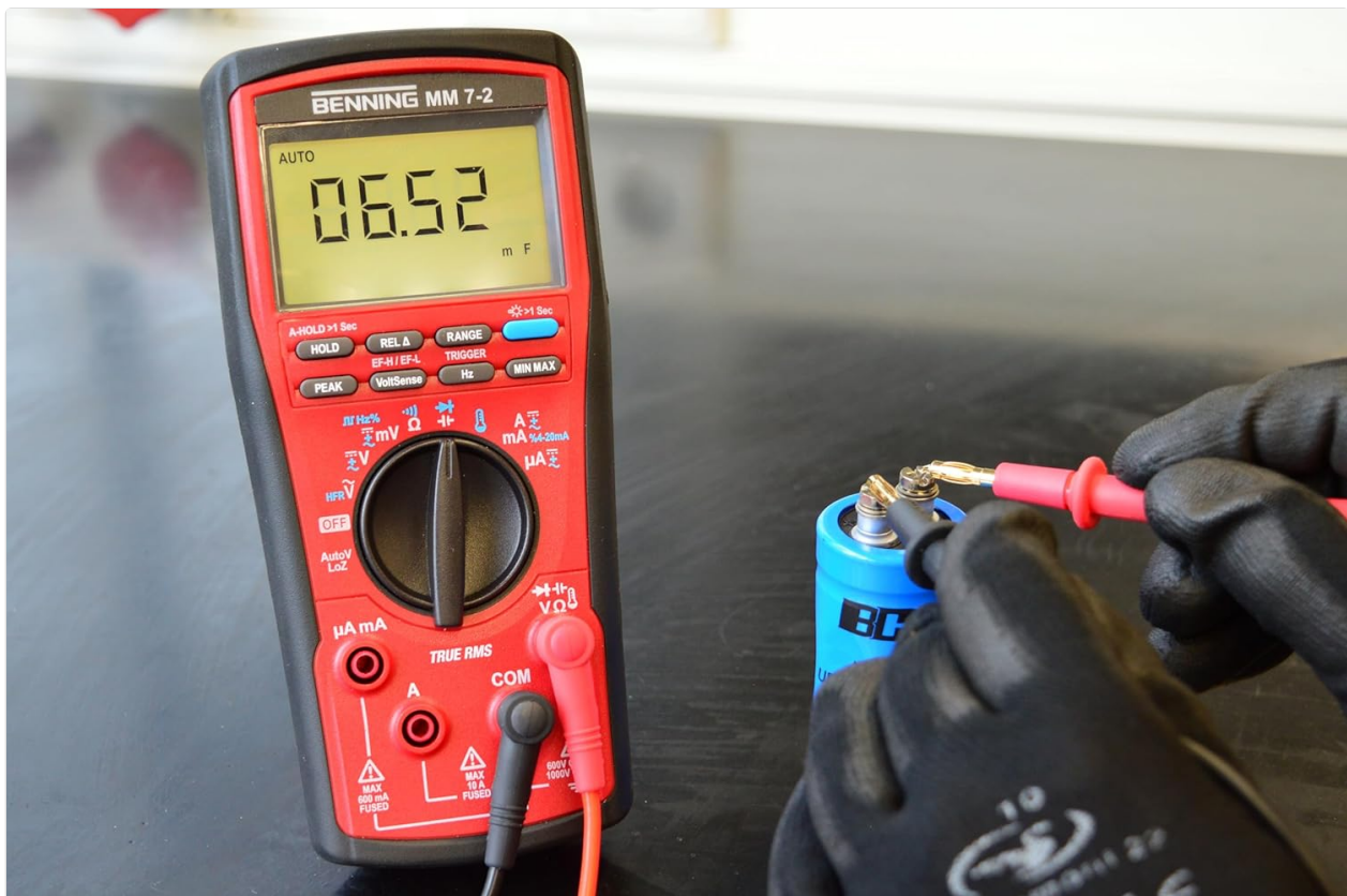
Figure 5: The BENNING MM 7-2 Multimeter accurately measuring the capacitance of a large blue electrolytic capacitor, illustrating its capability for component analysis.
