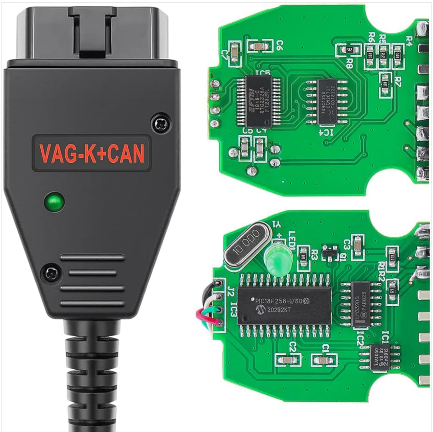
Image: The PARANNIC OBD2 K+CAN Commander 1.4 device, illustrating its OBD2 connector and the internal circuit board components, including the FTDI chip.
