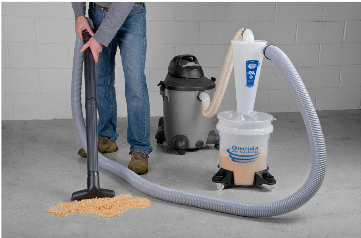
Figure 5: The clear collection bucket of the Dust Deputy 2.5 Deluxe, showing accumulated sawdust.
