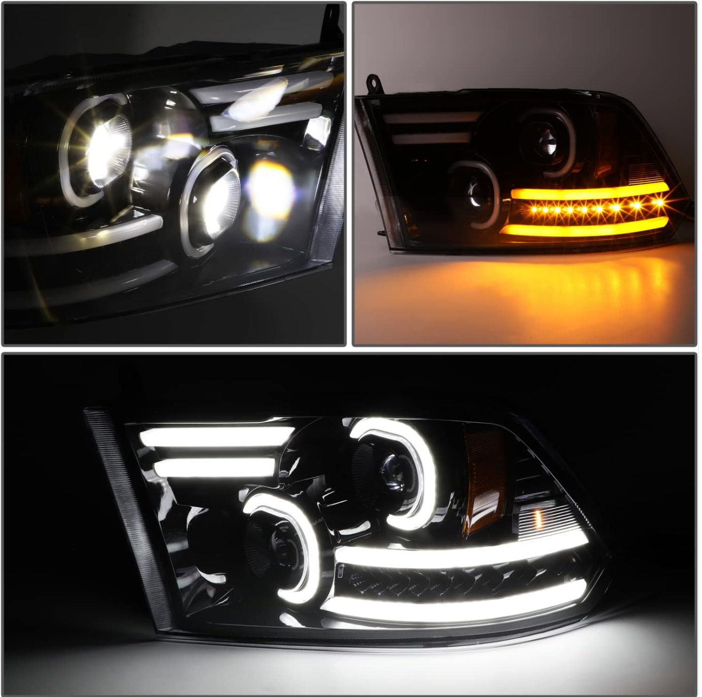
Image 6.1: The headlights displaying their various light functions, including the bright white DRLs and the amber sequential turn signals.
