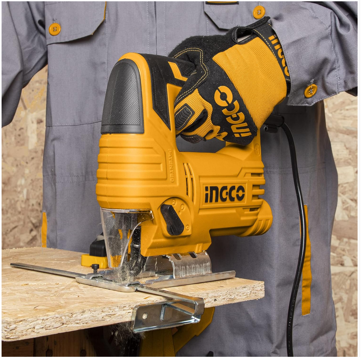
Figure 5.4: Proper grip and positioning of the jigsaw during operation on a wooden workpiece.
