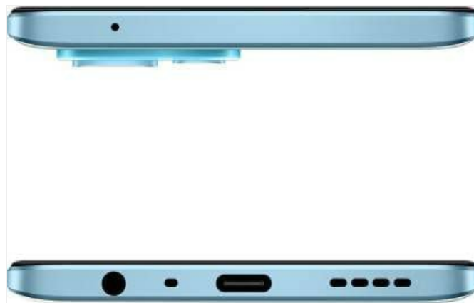
Figure 2: Top and bottom edges of the device. The bottom edge features the USB Type-C port, speaker grille, and microphone. The top edge includes a secondary microphone.
