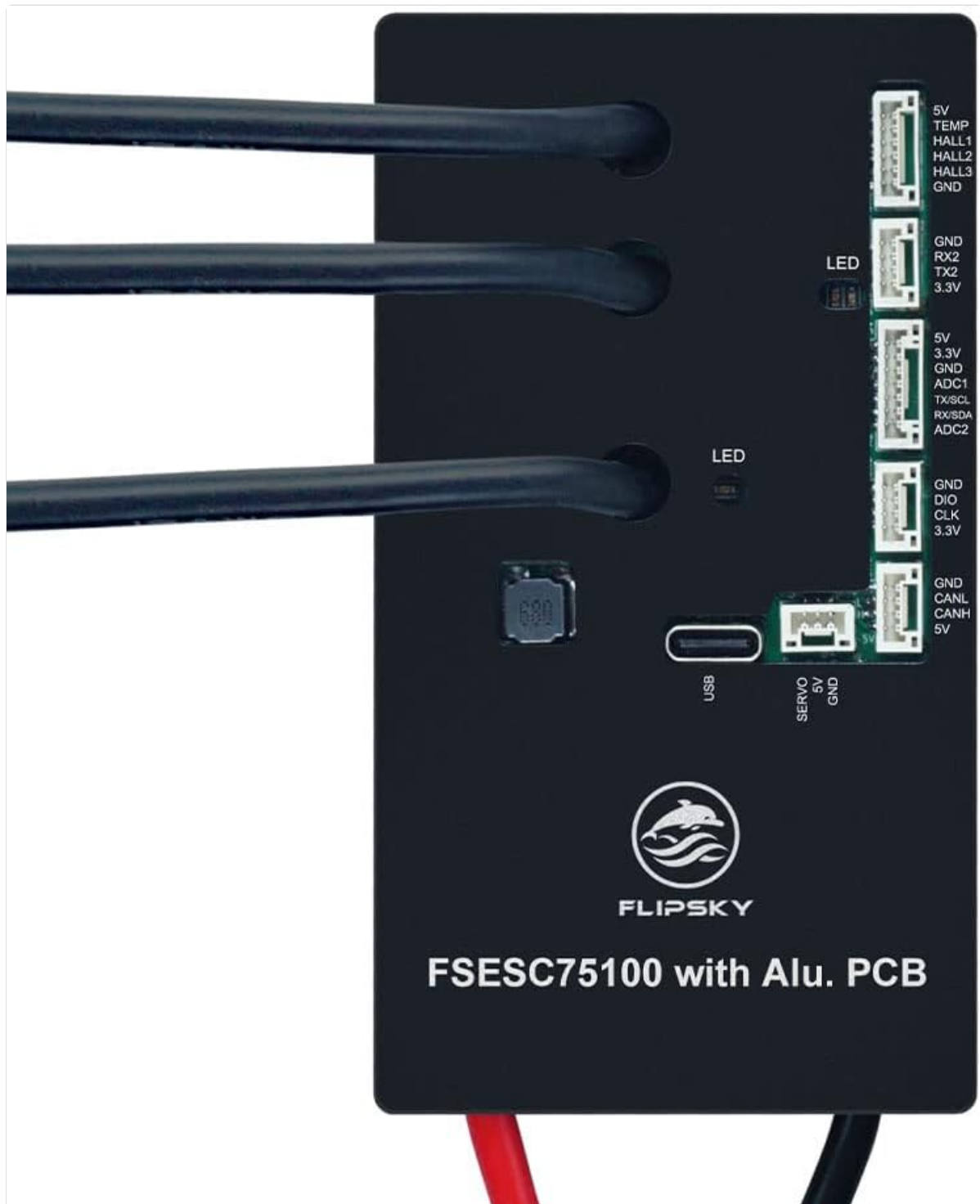
Image: Front view of the FLIPSKY FSESC75100, showcasing its compact design and main connections.
