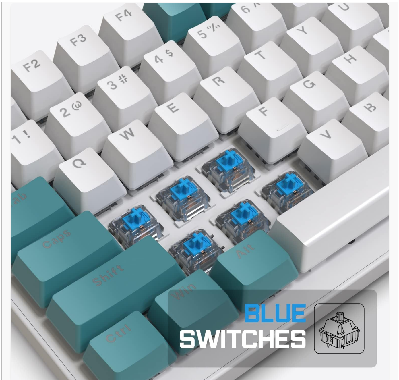
Image 4.1: A close-up view of the blue mechanical switches, known for their tactile feedback and audible click, which are featured in the ZIYOU LANG K3 keyboard.
