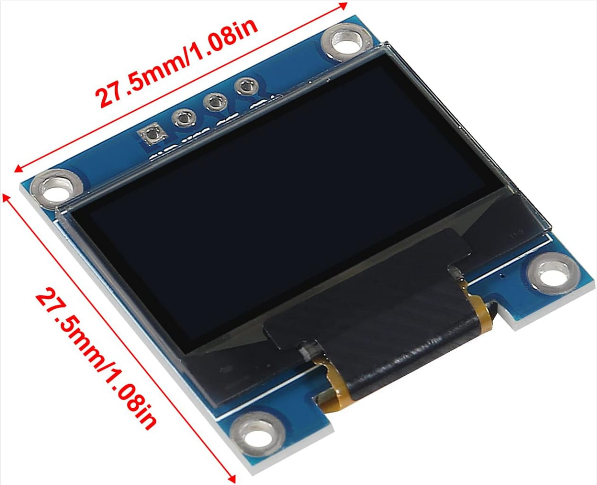
Image 2.1: Physical dimensions of the 0.96 inch OLED module, showing approximate measurements of 27.5mm x 27.5mm.
