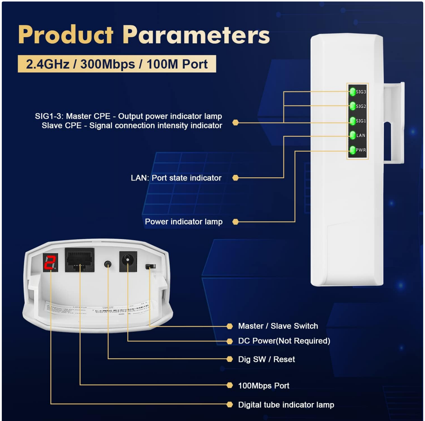
Image: A detailed view of the Binardat Wireless Bridge, highlighting its ports (100Mbps Ethernet, DC Power, Dig SW/Reset) and LED indicators (SIG1-3, LAN, PWR, Digital Tube).
