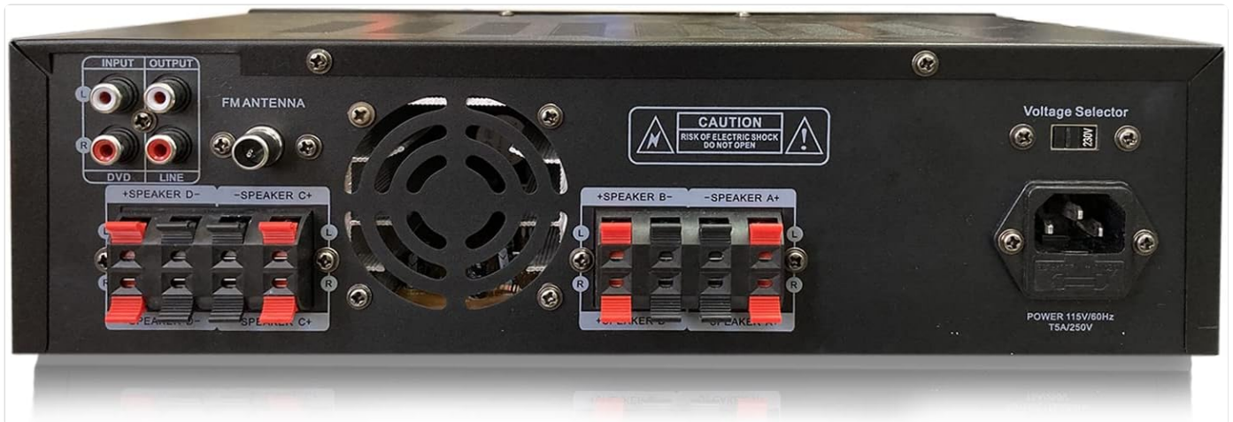
Figure 4.1: Rear Panel of the TPRX4CH Receiver
