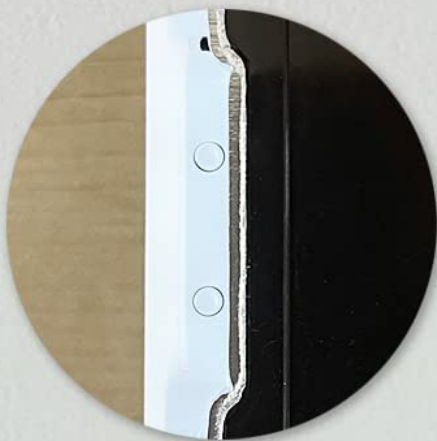
Figure 5: Trim buttons for sensitivity adjustment located under the cover plate.
