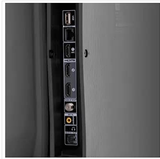
Image: Close-up view of the input/output ports on the back of the TCL 55A441 Smart TV. Ports include USB, Ethernet, multiple HDMI inputs, Cable/Antenna, AV In, and Optical Audio Out.
