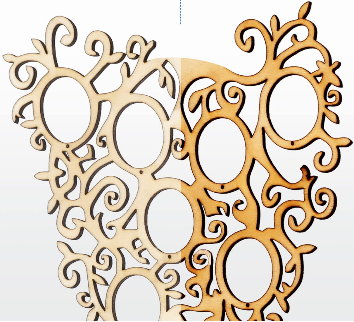
Image 5.2: A visual comparison demonstrating the improved cut quality achieved with air assist versus without.
