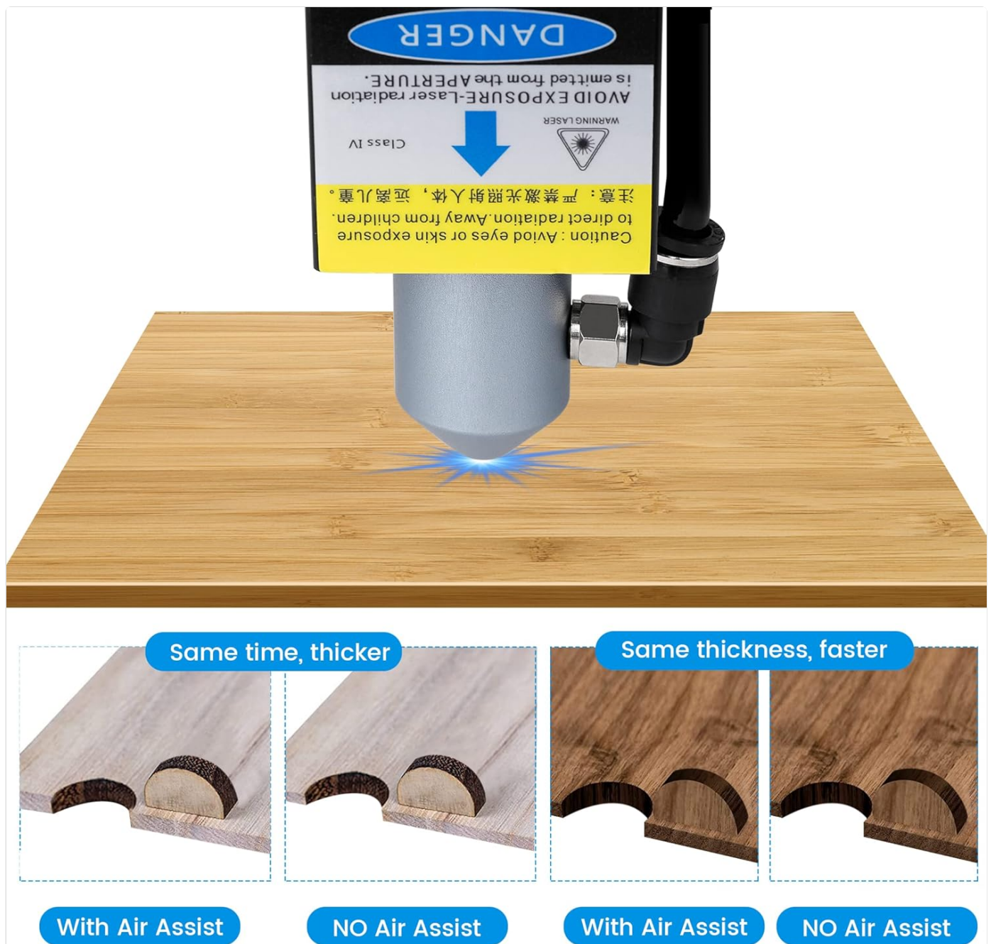
Image 5.3: Illustrates how air assist contributes to achieving thicker and faster cuts compared to operations without it.
