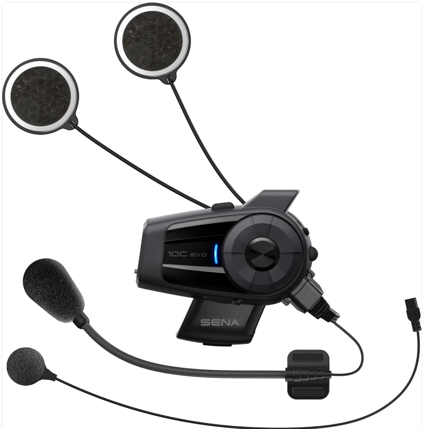
Image: A detailed view of the two microphone options: a flexible boom microphone with a foam cover and a smaller wired microphone, both designed for helmet integration.
