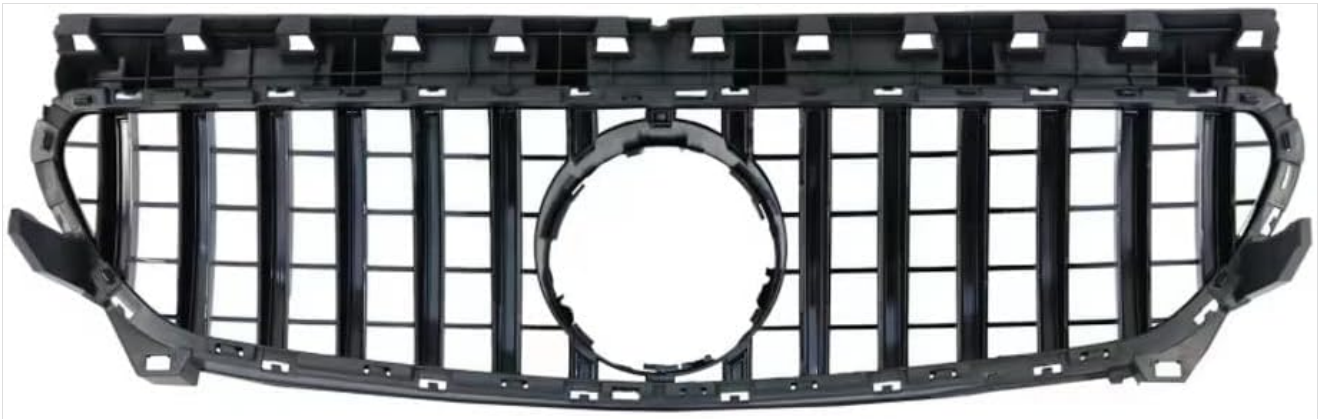
Image 2.2: Rear view of the grille, illustrating the strong clips and tabs designed for secure mounting.
