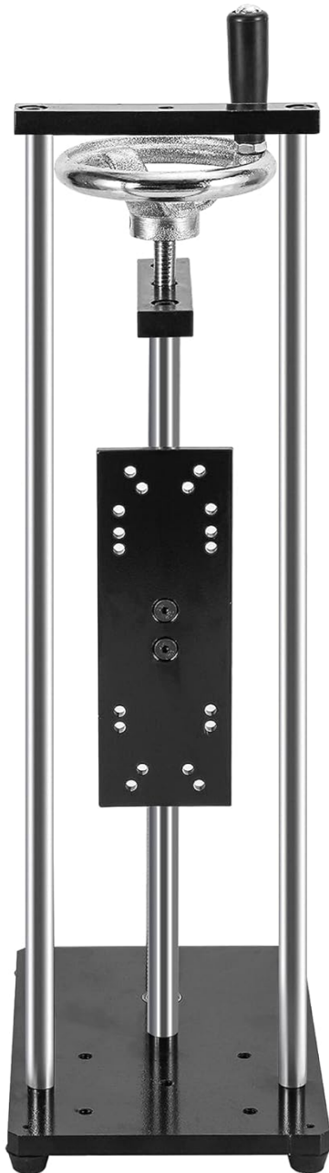
Figure 4.2: APH Test Stand Mounting Holes. This image highlights the mounting plate of the APH Test Stand, detailing the various hole patterns and their dimensions: 30x145mm, 40x100mm, 20x130mm, and 40x90mm. These patterns allow for versatile attachment of different force gauges.
