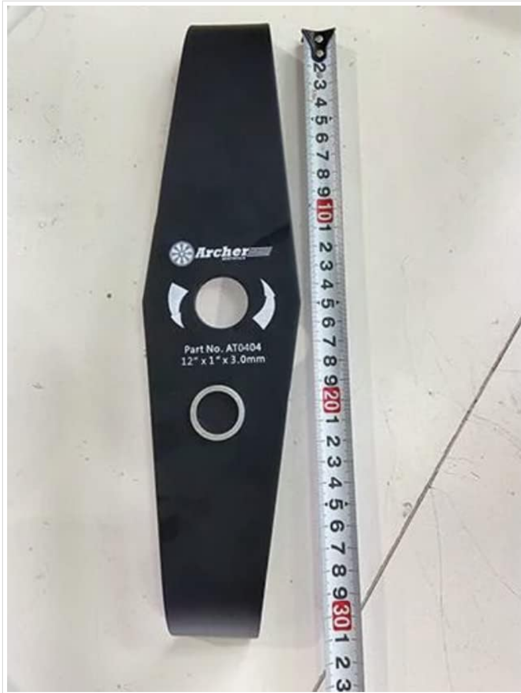
Figure 2: The Archer AT0404 3mm blade displayed next to a measuring tape, indicating its length and thickness. The blade is marked with "Archer", "Part No. AT0404", and dimensions "12" x 1" x 3.0mm".
