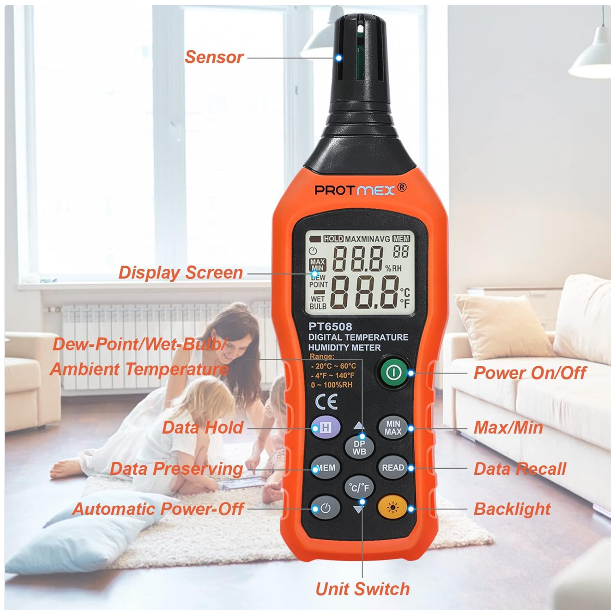
Figure 3: Key components and buttons of the PT6508.
