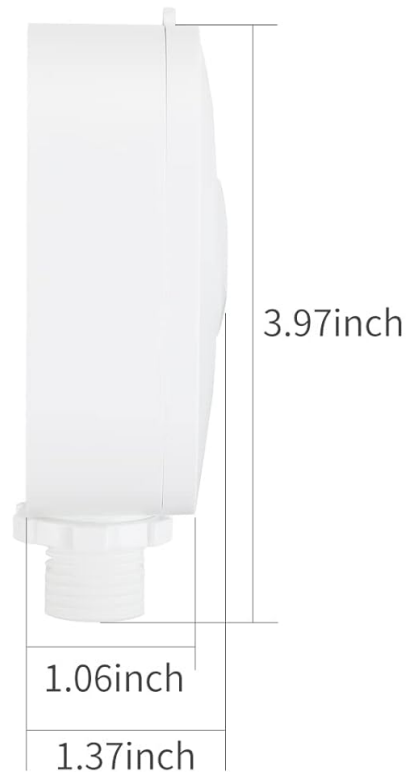
Figure 3: Dimensional drawing of the ECOELER YM2511 sensor. This diagram provides precise measurements of the sensor unit, including its length, width, and height, along with the diameter of the threaded conduit.
