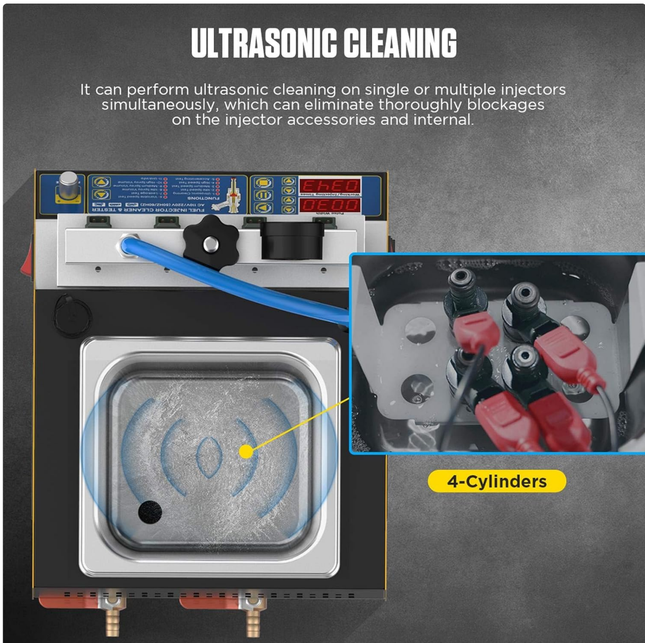
Figure 4: Ultrasonic cleaning process in the unit's bath.
