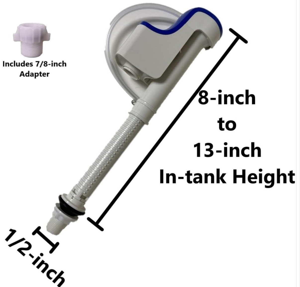
Figure 2.2: This image illustrates the adjustable height range of the NuFlush fill valve, from 8 to 13 inches, and highlights the 1/2-inch connection size. It also shows the optional 7/8-inch adapter.
