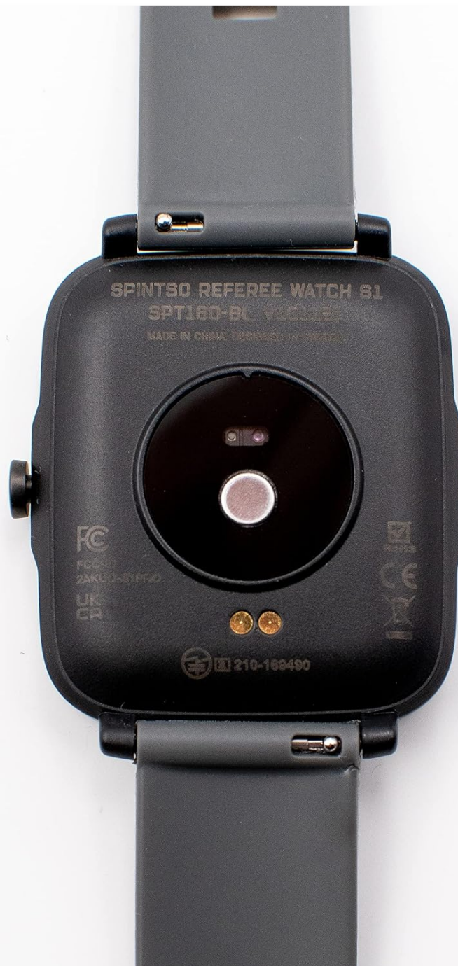
Image: The back of the SPINTSO S1 smartwatch, showing the optical heart rate sensor and charging contacts.
