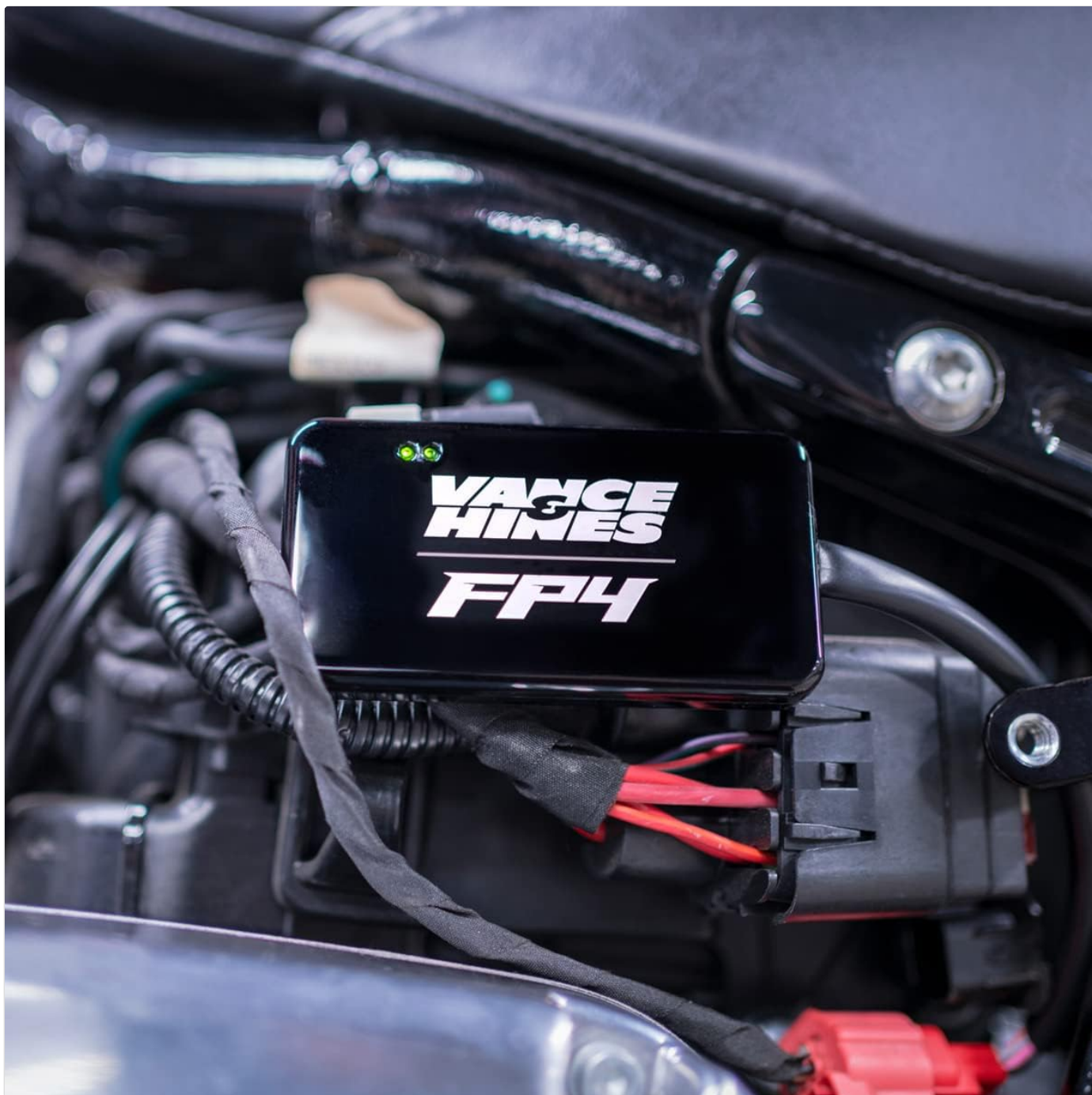
Figure 4: A close-up view of the FP4 module securely connected to the motorcycle's electrical system, indicating proper installation.
