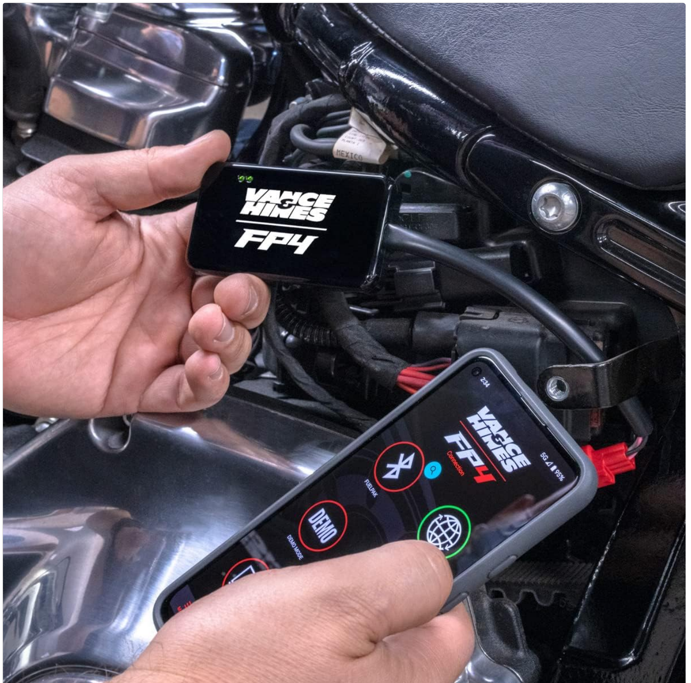
Figure 3: Illustrates the process of connecting the FP4 device to the motorcycle's diagnostic port, showing the secure fit of the harness.
