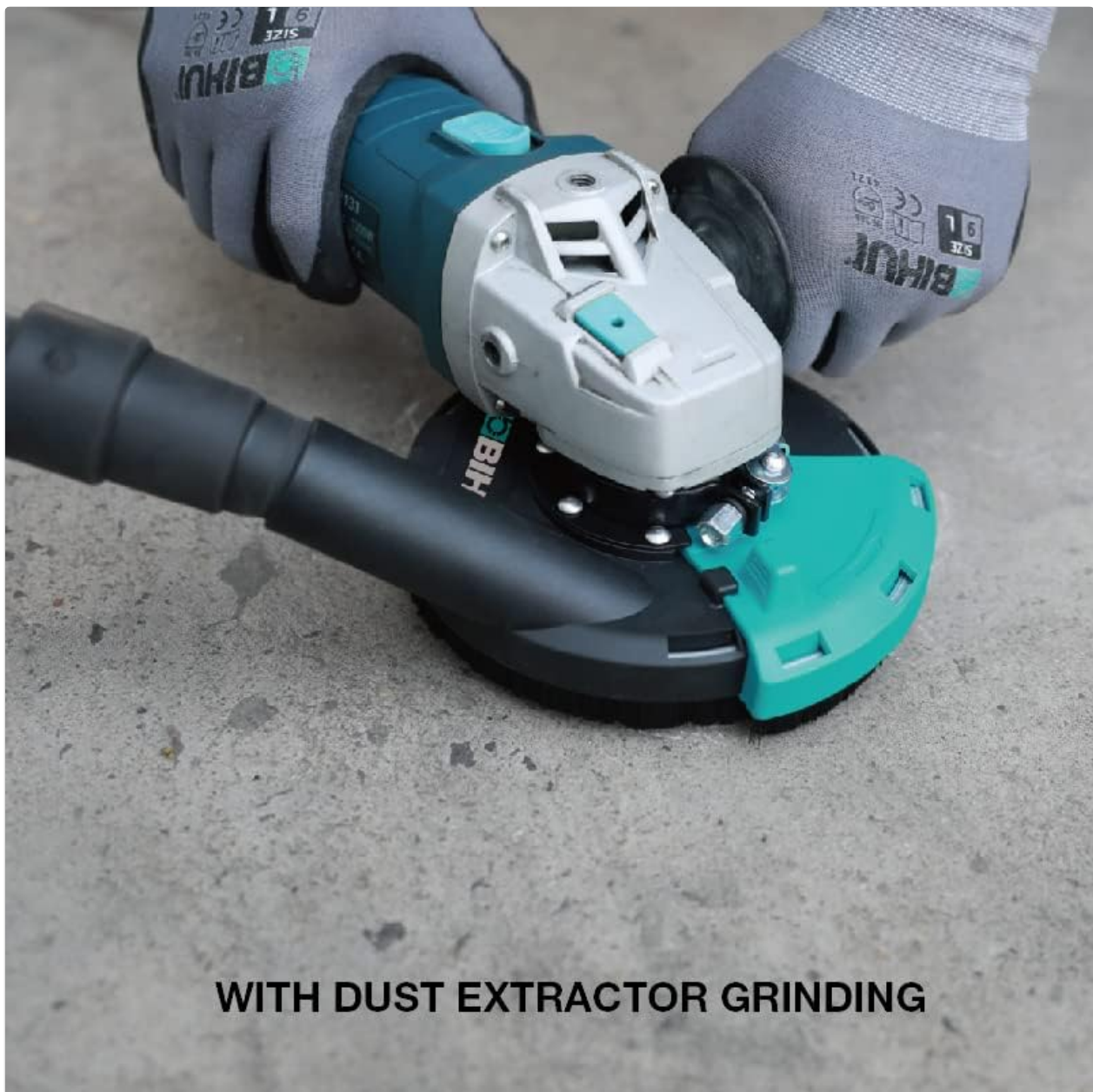
Figure 5.2: Grinding with the BIHUI dust extractor, demonstrating effective dust containment and a cleaner work area.
