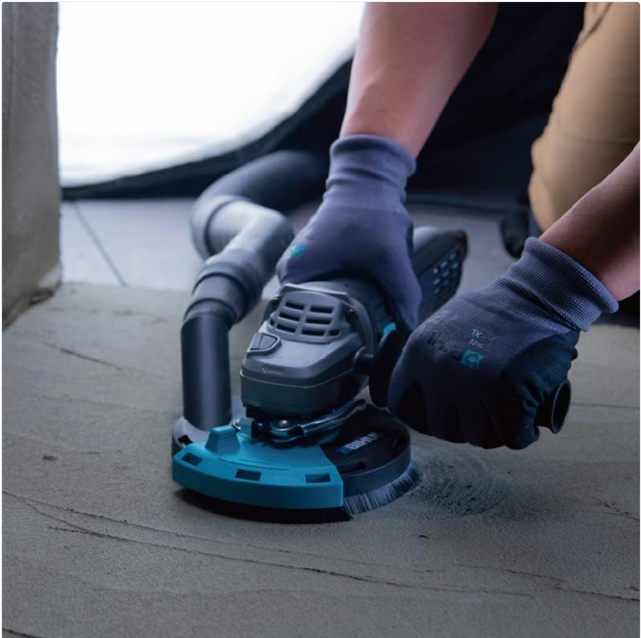
Figure 4.1: The dust extractor securely attached to an angle grinder, ready for vacuum connection.
