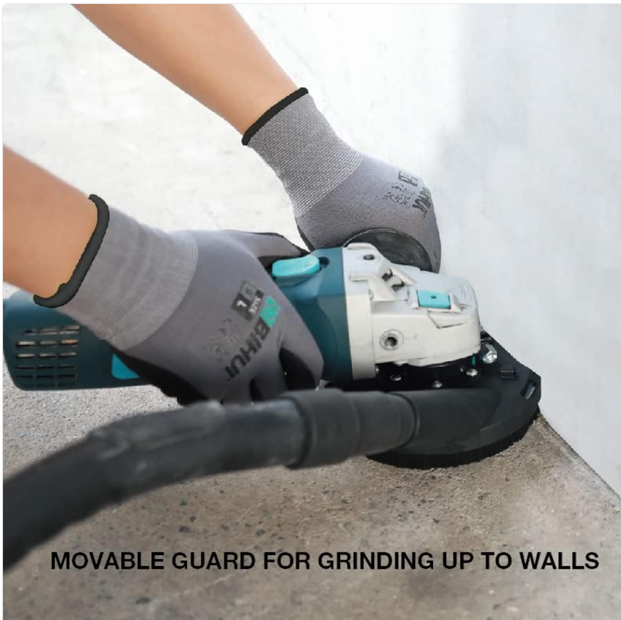
Figure 5.4: The movable guard allows for efficient grinding up to walls and edges, maximizing dust collection in tight spaces.
