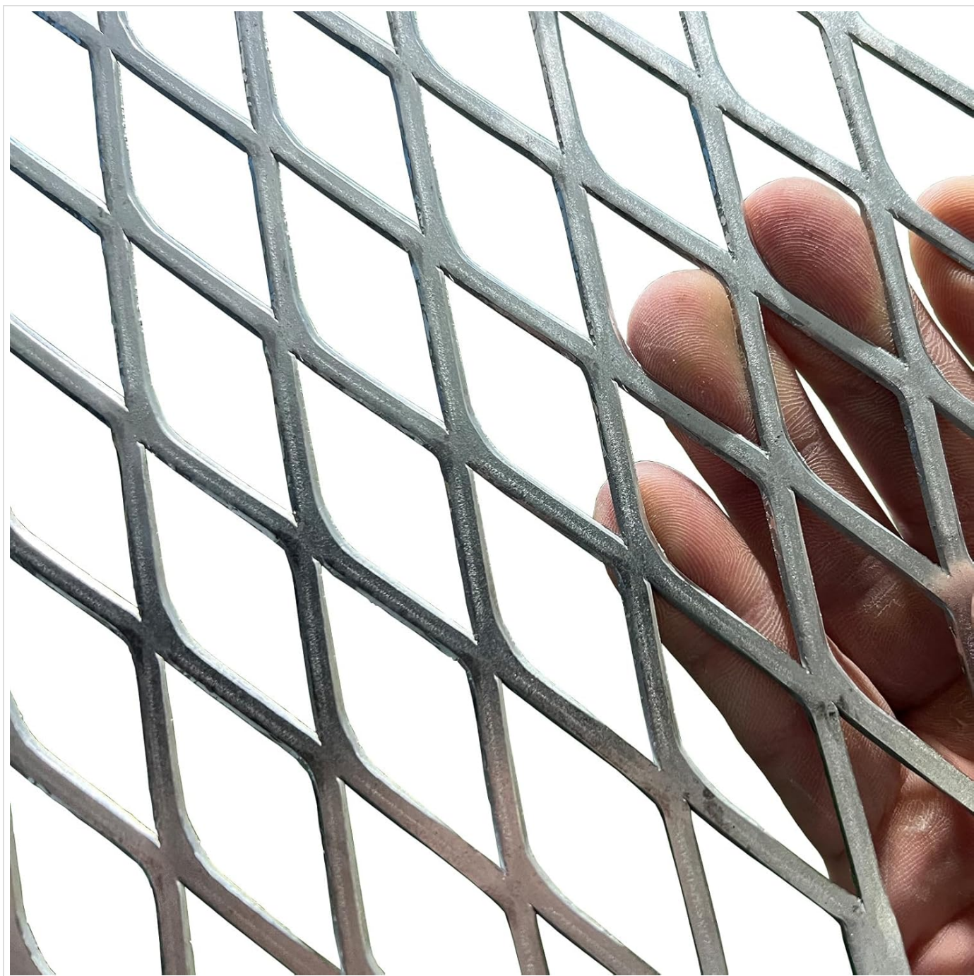
Figure 1: Close-up of the expanded metal mesh, showing the diamond pattern and the thickness of the material. A hand is visible behind the mesh, demonstrating the open structure.
