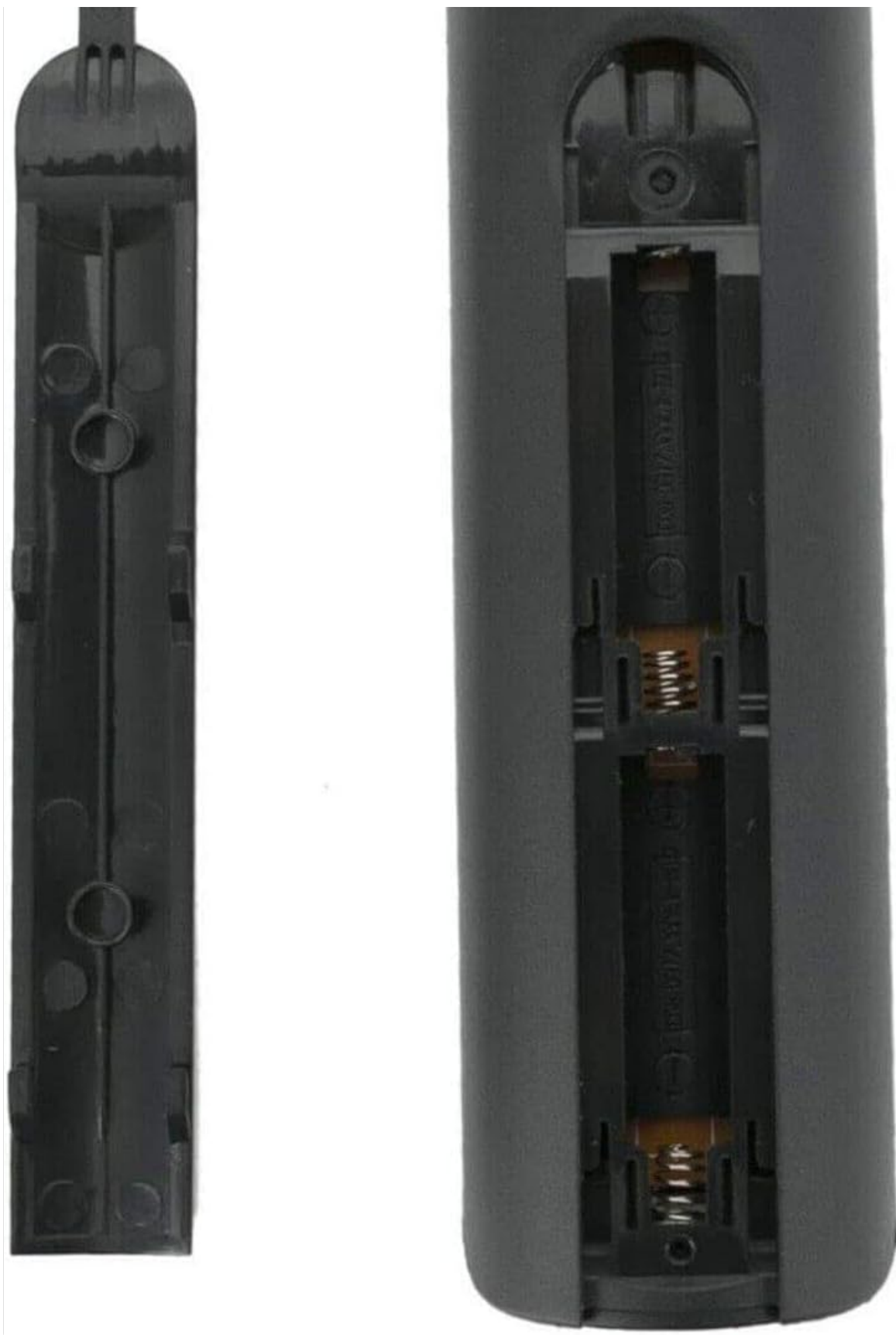
Figure 1: Battery compartment with two AAA batteries. Ensure correct polarity when inserting batteries.
