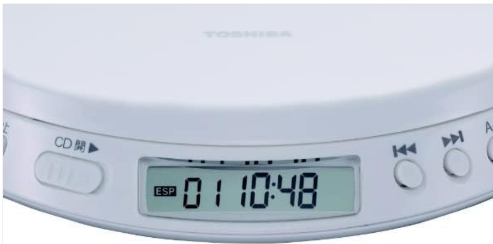
Figure 4.2: Close-up of the player's front panel, featuring the LCD display and control buttons for playback, track navigation, and speed control.
