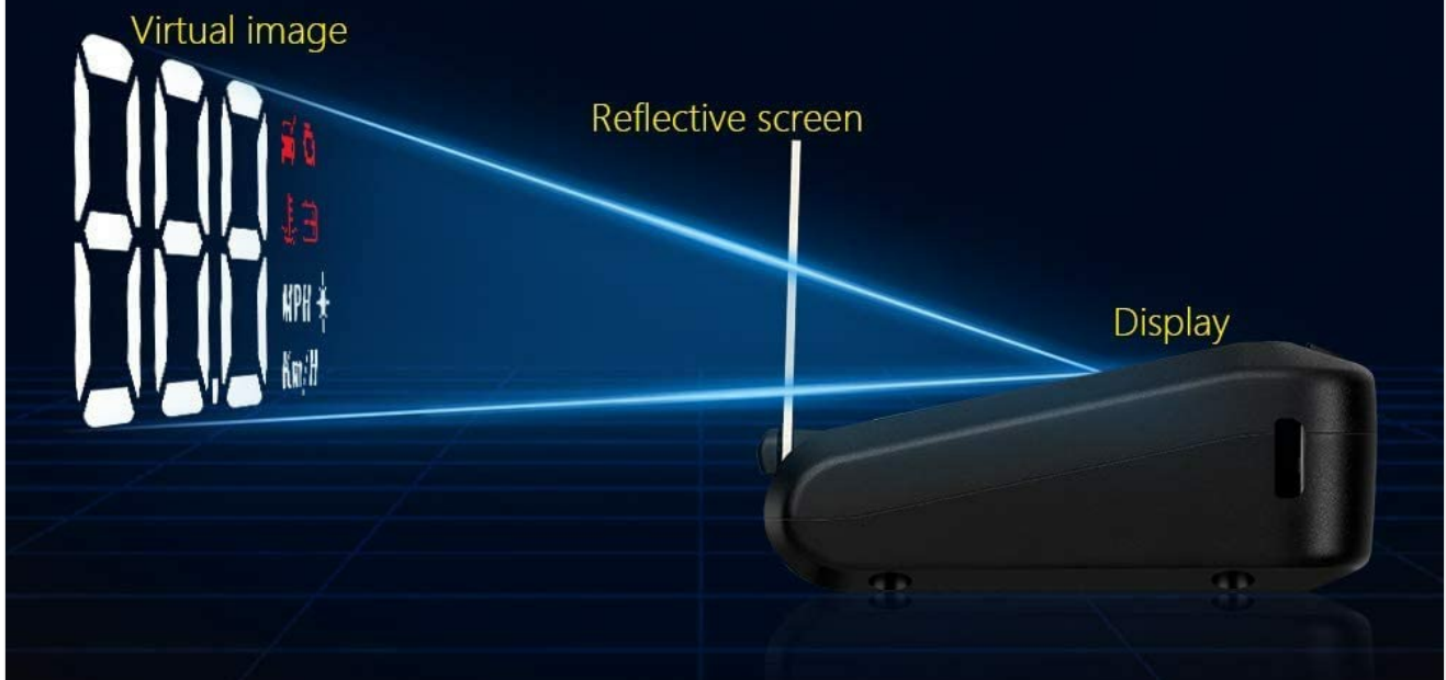
Image 4.1: Diagram explaining the levitate imaging principle for the HUD's display.
