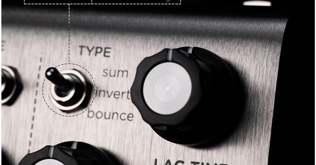
Figure 5: Detail of the Type switch for the Doubletracker side, providing Sum (decks in phase), Invert (Lag Deck phase inverted), and Bounce (Right Lag Deck bounced to left input for stereo ping-pong or mono double-echo).
