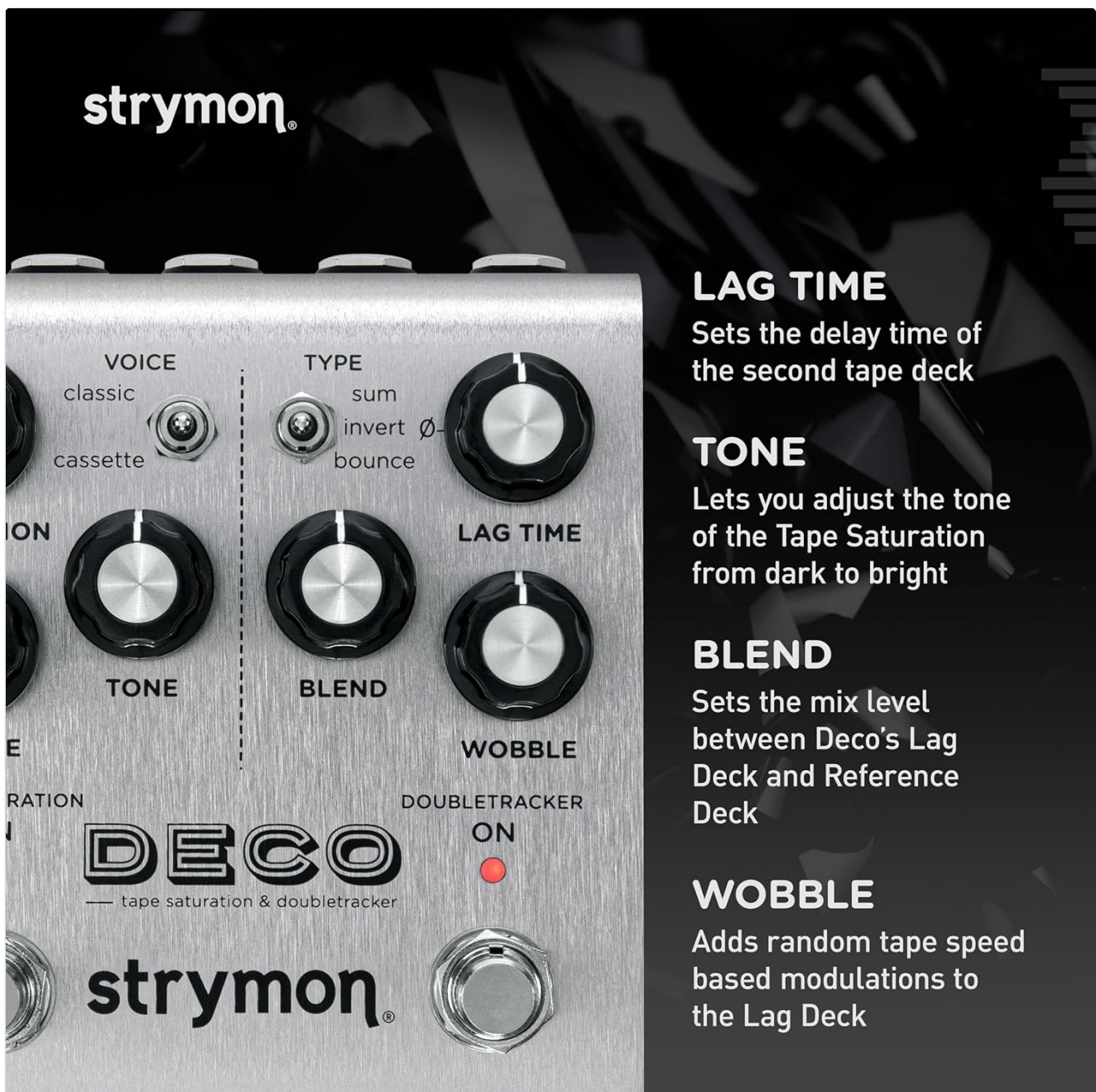
Figure 6: Key controls on the Deco V2. Lag Time sets the delay time of the second tape deck. Tone adjusts the tone of the Tape Saturation from dark to bright. Blend sets the mix level between Deco's Lag Deck and Reference Deck. Wobble adds random tape speed based modulations to the Lag Deck.
