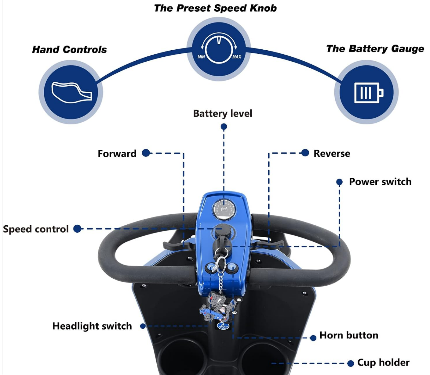
Figure 3.2: Detailed view of the scooter's intuitive controls, including the preset speed knob, hand controls, battery gauge, forward/reverse switch, power switch, headlight switch, horn button, and cup holder.
