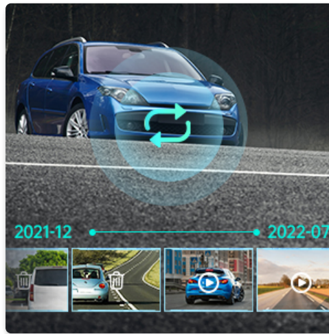
Figure 4.3: Loop recording ensures continuous operation by overwriting the oldest files.
