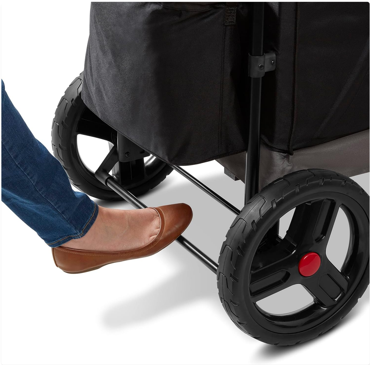
Image 2.2: Demonstrating the use of the rear foot brake for securing the wagon in a stationary position.
