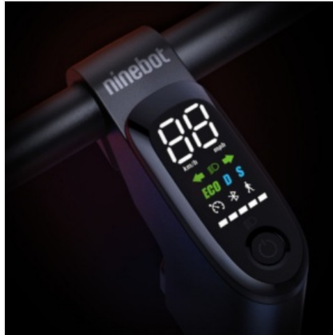
Figure 3: The digital dashboard displays speed, battery status, and selected riding mode (ECO, D, S).
