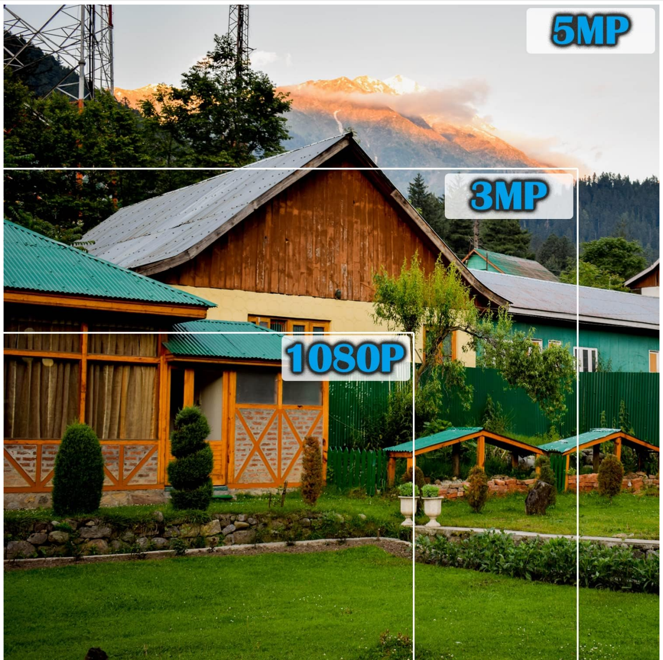
Figure 2.3: Visual comparison of 5MP, 3MP, and 1080P resolutions, demonstrating the superior detail of 5MP.
