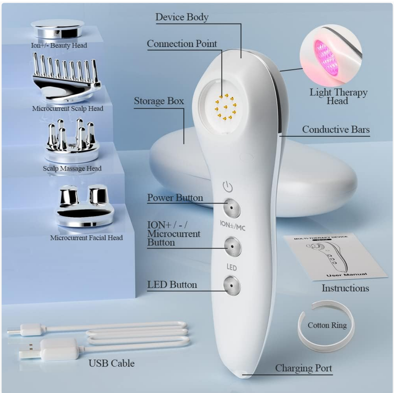
Image 2.1: Labeled diagram of the device, showing the main body, interchangeable heads (Ion+/- Beauty Head, Microcurrent Scalp Head, Scalp Massage Head, Microcurrent Facial Head), control buttons (Power, ION+/-, LED), charging port, and accessories like the USB cable and cotton ring.
