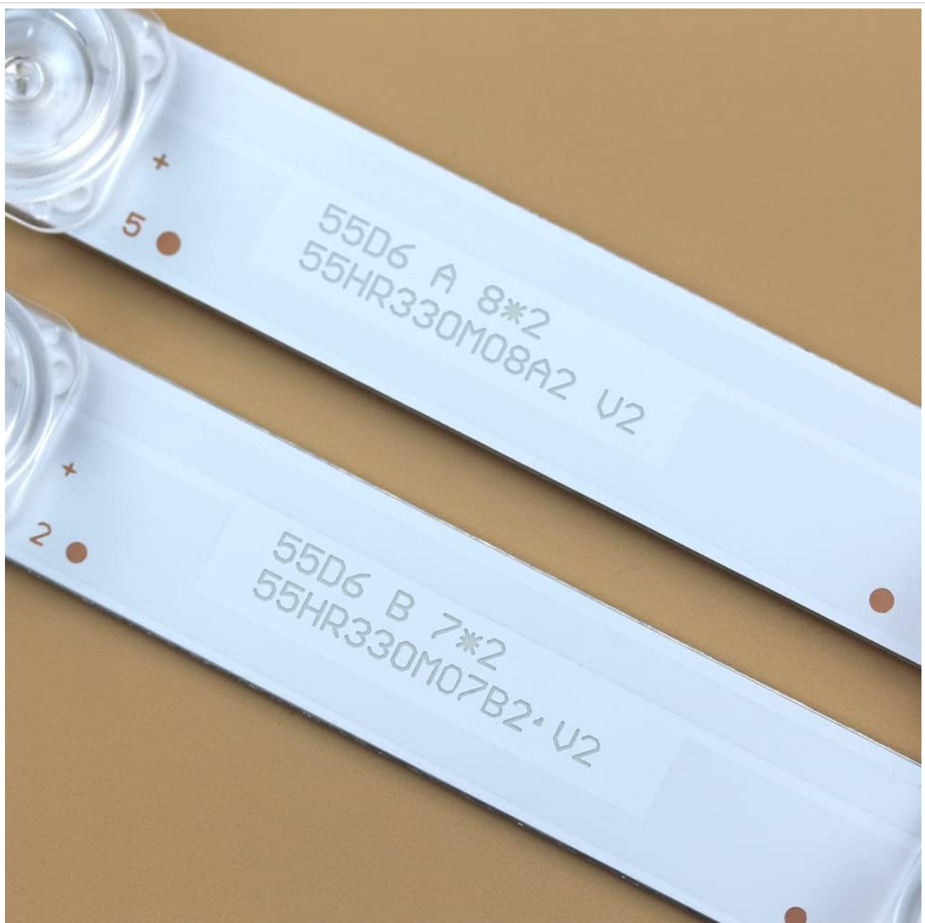
Figure 3.1: Example of part numbers printed on the LED backlight strips for identification.
