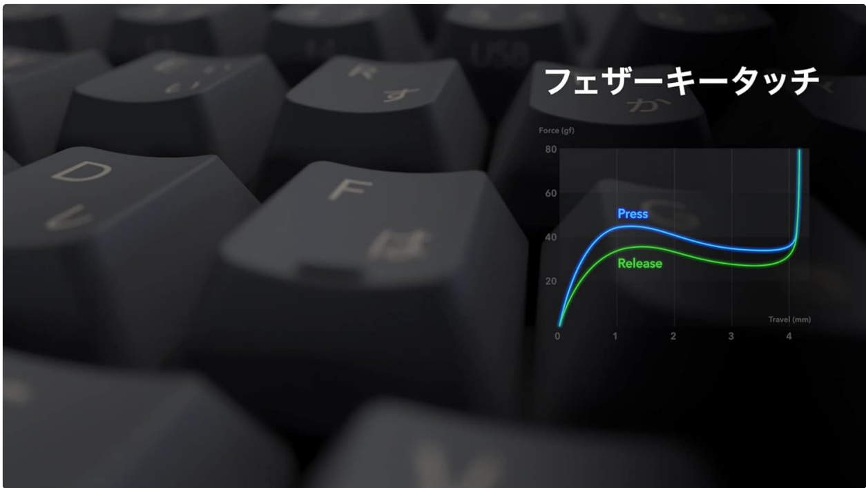
Image: A force curve graph demonstrating the press and release characteristics of Topre switches.
