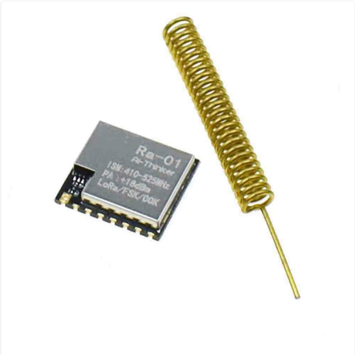
Figure 5.1: The Reland Sun RA-01 LoRa module shown with its accompanying 433MHz helical antenna. This image illustrates the compact size of the module and the typical antenna used for wireless communication.
