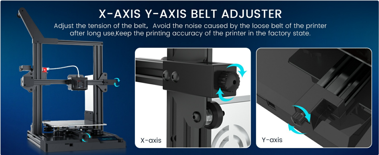
Image: Instructions for adjusting the X-axis and Y-axis belts to ensure optimal tension.
