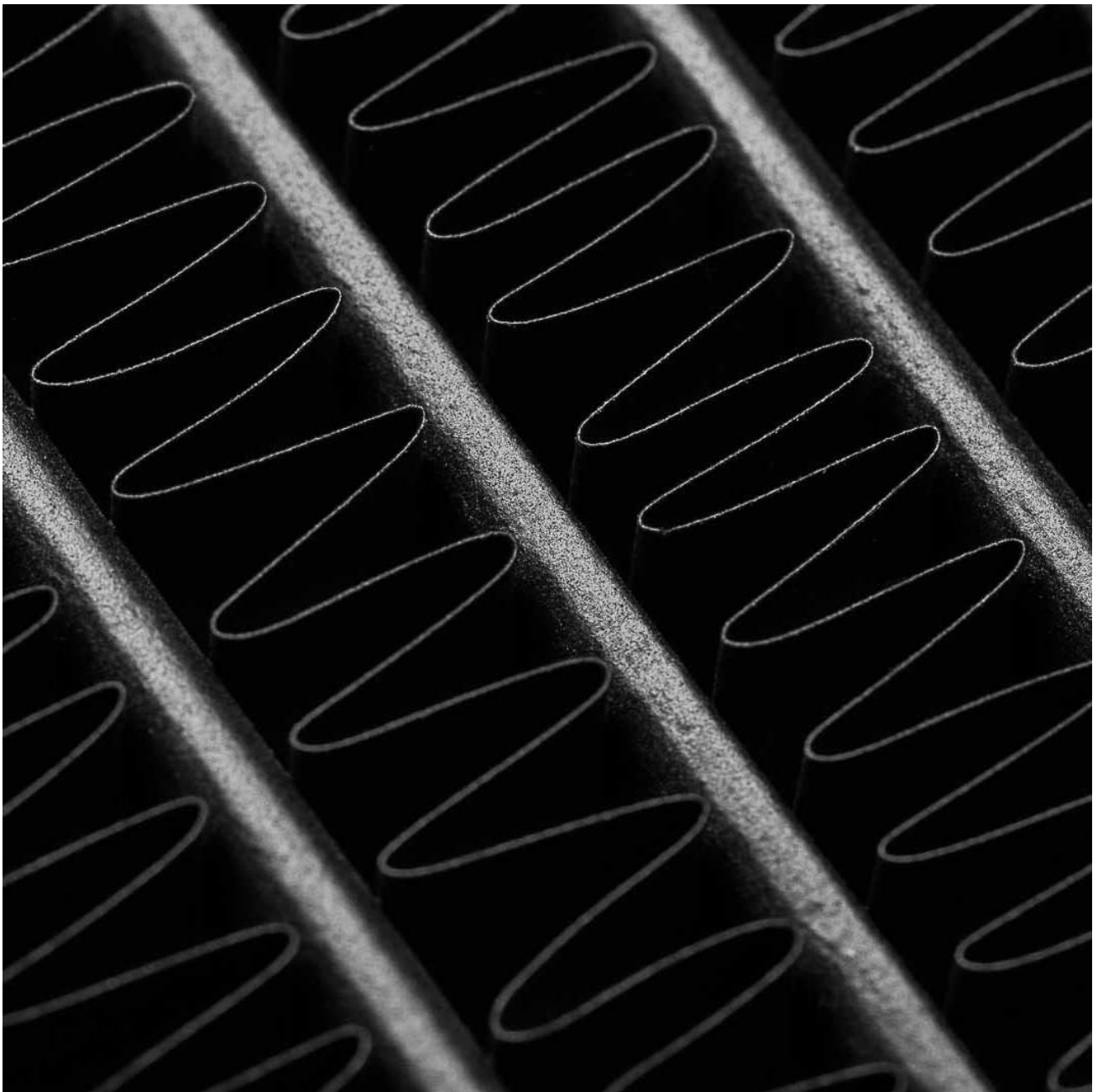
Figure 5.1: A close-up view of the radiator's copper fins, illustrating the 18 FPI density designed for efficient heat exchange.
