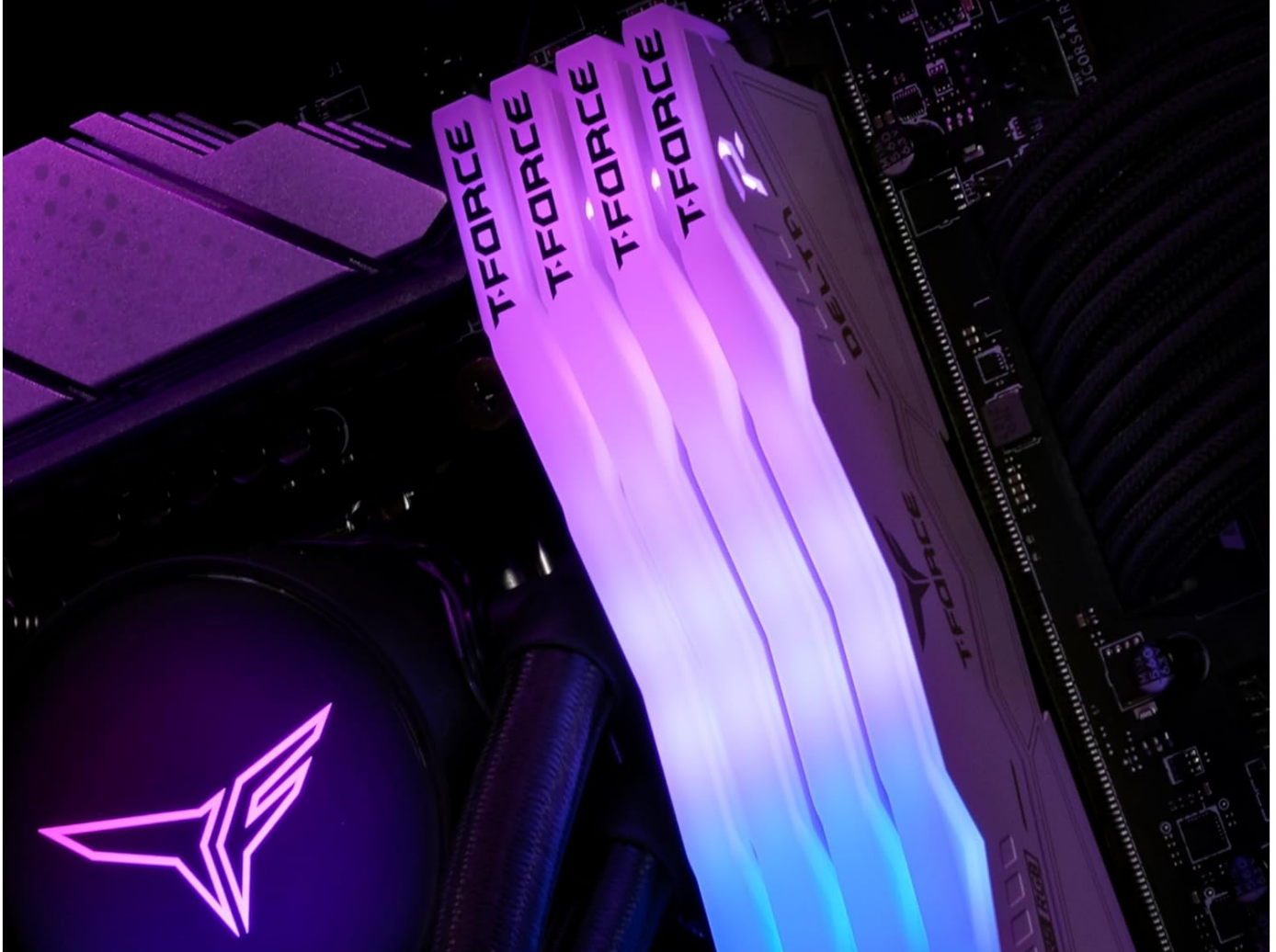
Figure 2.2: The RAM modules support Intel XMP 3.0 for one-click overclocking.
