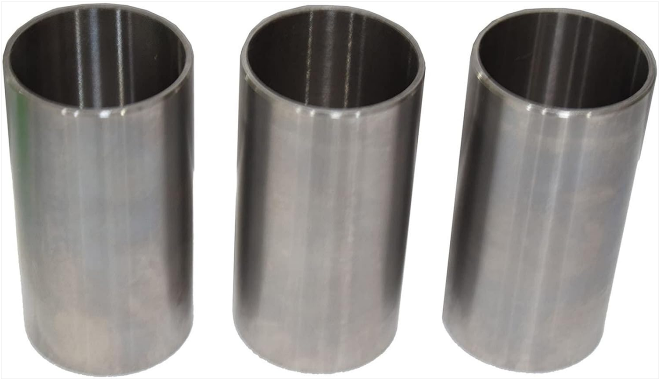
Figure 2.2: Close-up of the three semi-finished cylinder liners.
