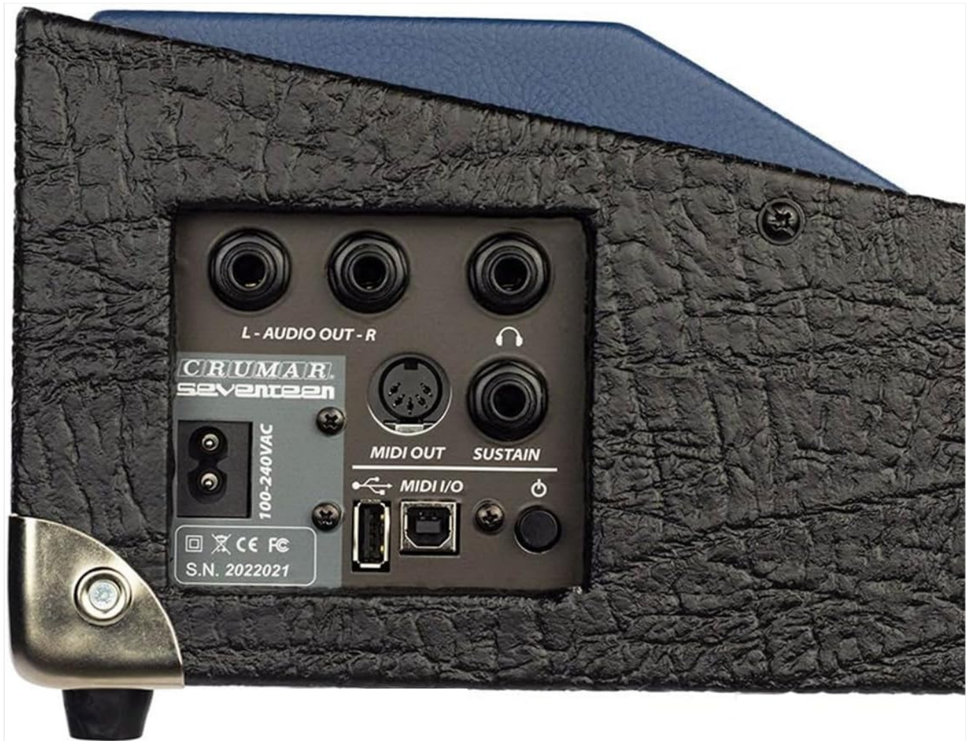
Figure 3: Rear panel of the Crumar Seventeen, showing power input, L/R audio outputs, headphone jack, MIDI I/O, and sustain pedal input.
