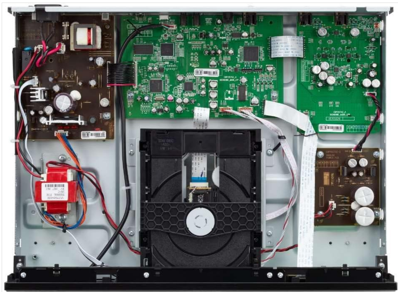
Image: Internal view of the Denon DCD-900NE, showing the organized layout of components, including the disc drive and circuit boards, designed for vibration resistance.
