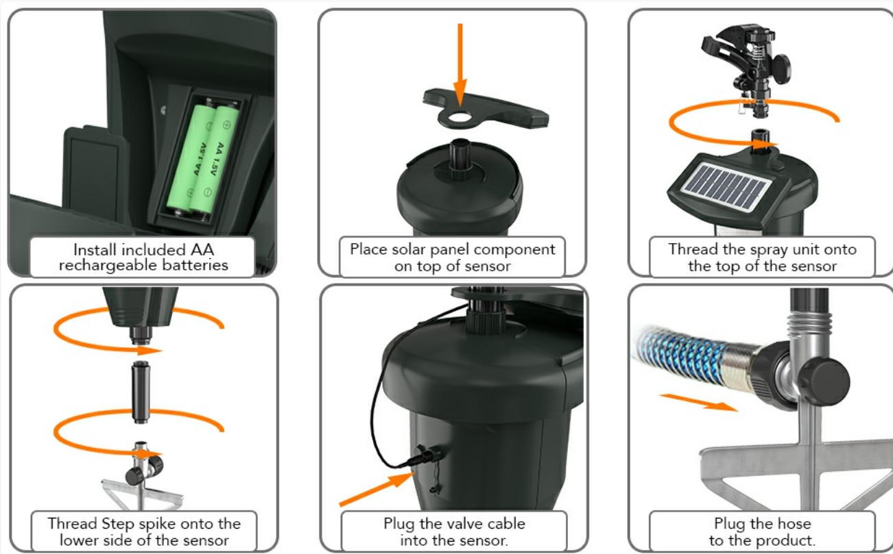
Image: Visual guide illustrating the six steps for assembling and connecting the animal repeller device.
