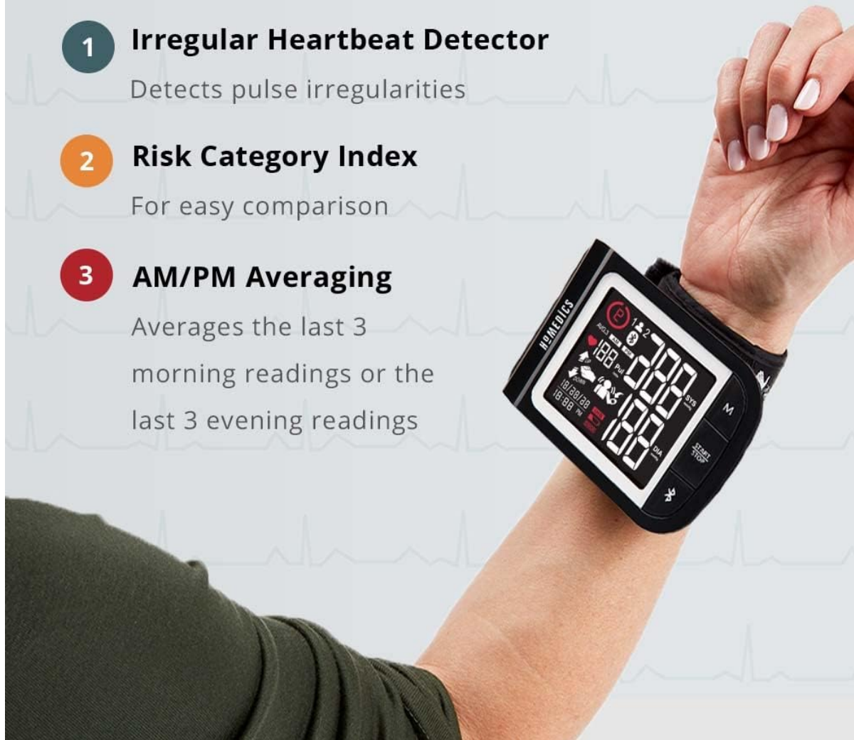
Image: The monitor's display highlighting the Irregular Heartbeat Detector symbol, the Risk Category Index bar, and the AM/PM averaging indicator.
